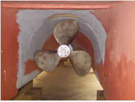
The propeller is protected by a tunnel, shown in the two images above
