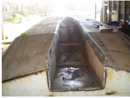
The propeller is protected by a tunnel, shown in the two images above
