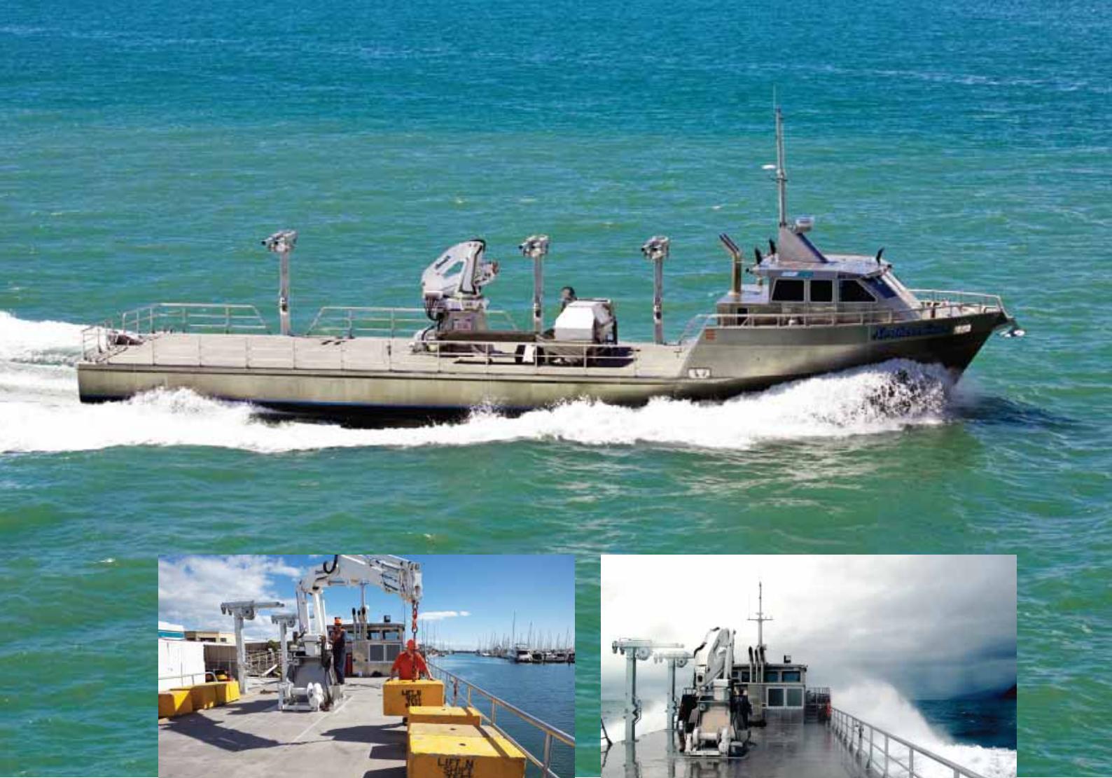
Northern Quest is stable and designed for 100 tonne deck loads in all weather
