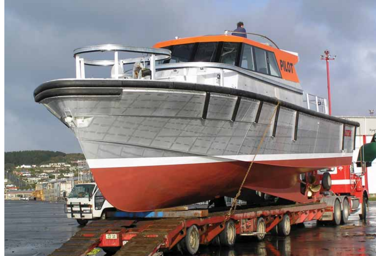
Takitimu II shows her underwater configuration with twin skegs
