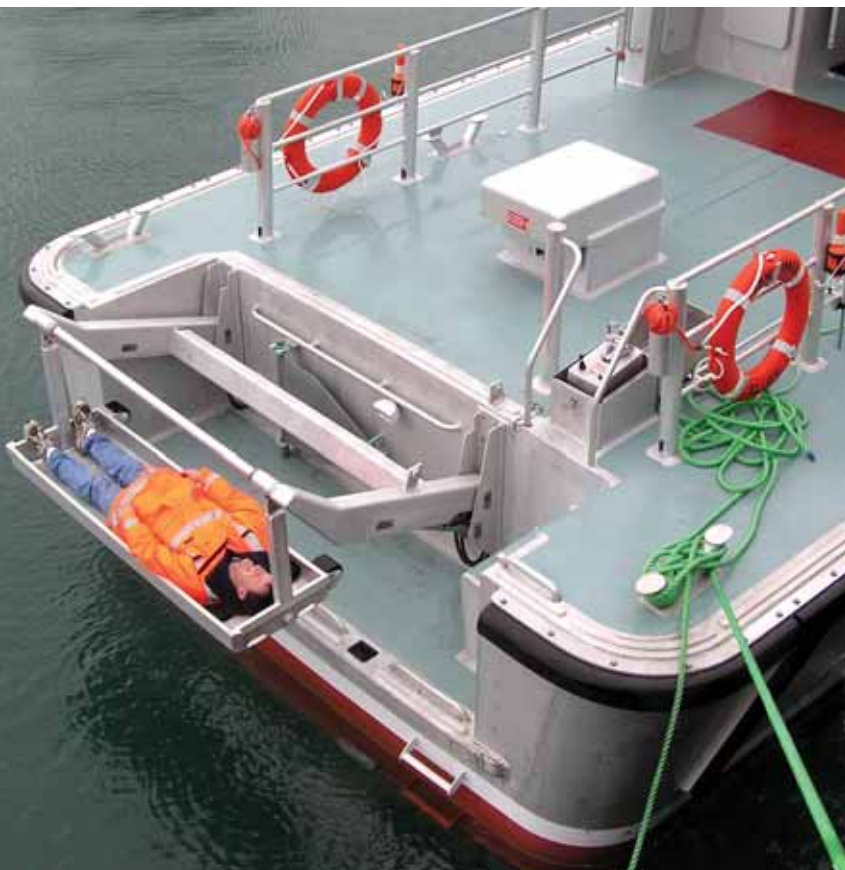
The unique man-overboard recovery system
